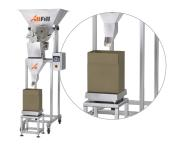
E/SERIES GROSS SERIES: Also available is the 101e with platform scale for bulk fill applications.
